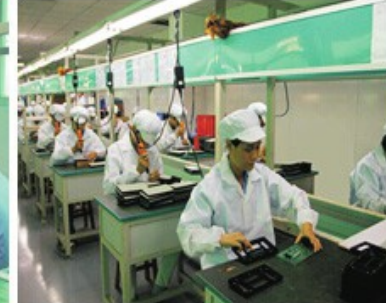
Fix mask and external parts to module
