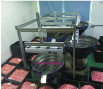
Mixing leds to ensure the same lumens for every led lamp
