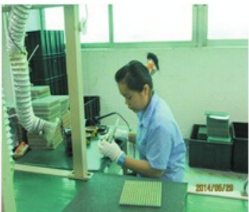
Check whether the leds well soldering or not. Check piece by piece.
