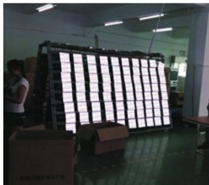
Every module should be tested for 48 hours before assembly
