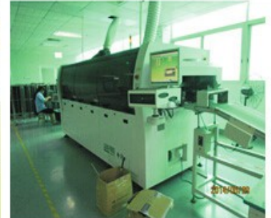
Wave-soldering and reflow-soldering to fix IC onto PCB board
